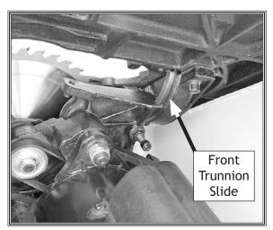
**Figure 83.** Trunnion slide (front slide shown)
